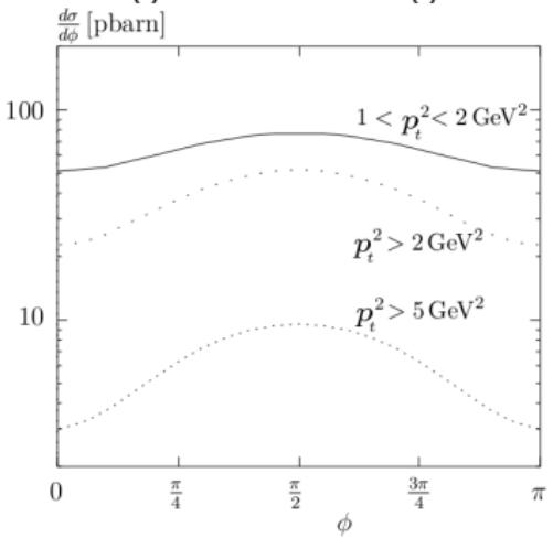
$$d\sigma/d\phi \propto 1 + A \cos(2\phi)$$
